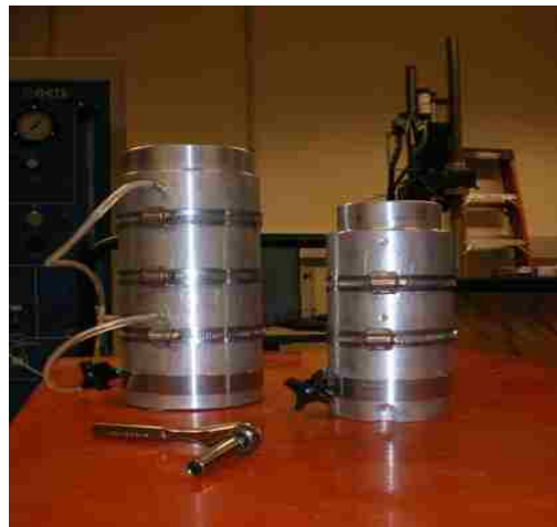
Figure 3.4 Split Molds Used for Compaction
