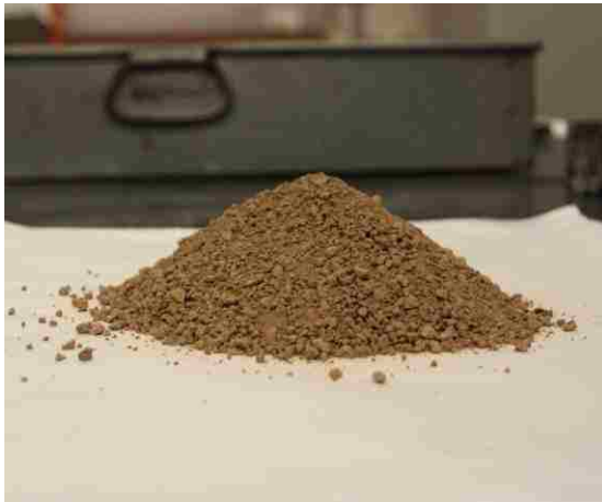
Figure 3.2 Processed A-6 and A-7-6 Soil Passing U.S. No. 4 Sieve
