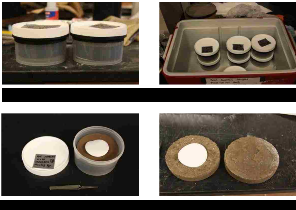
Figure 3.12 Soil Suctions Measurement with Filter Paper Method
