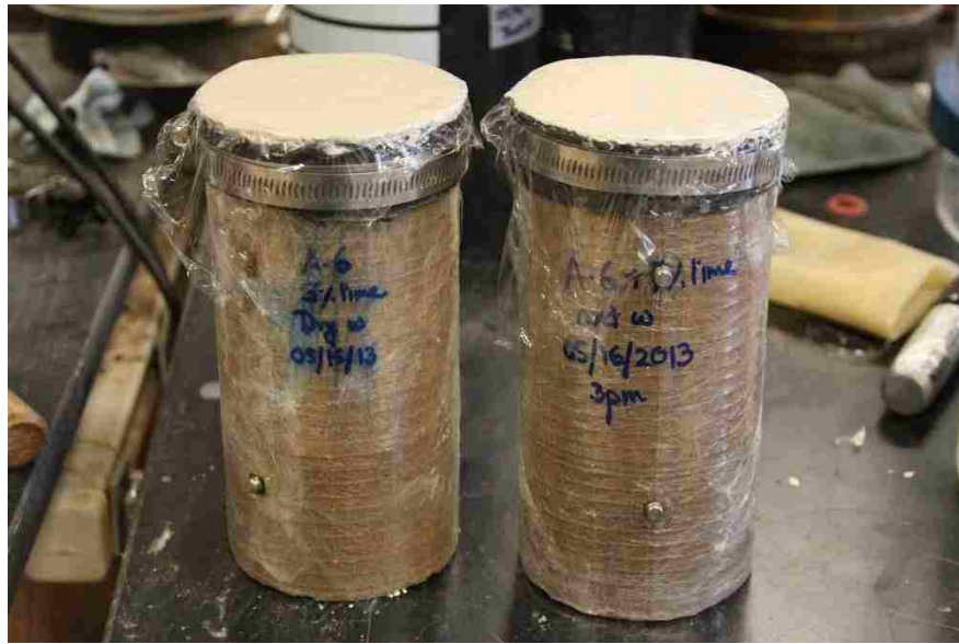
Figure 3.7 Capped Plastic Wrap Subgrade Samples
