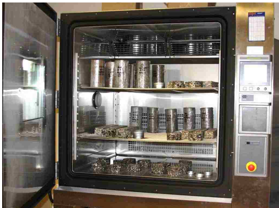
Figure 3.15 Samples in Freeze-Thaw Chamber subjected to F-T cycles
