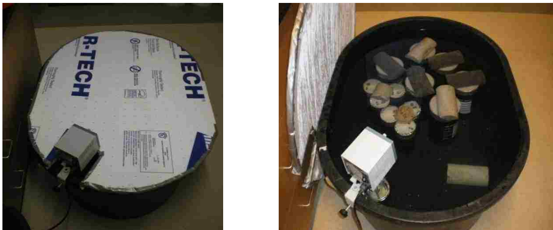
Figure 3.6 Stabilized Subgrade Soil in the Curing Tank
